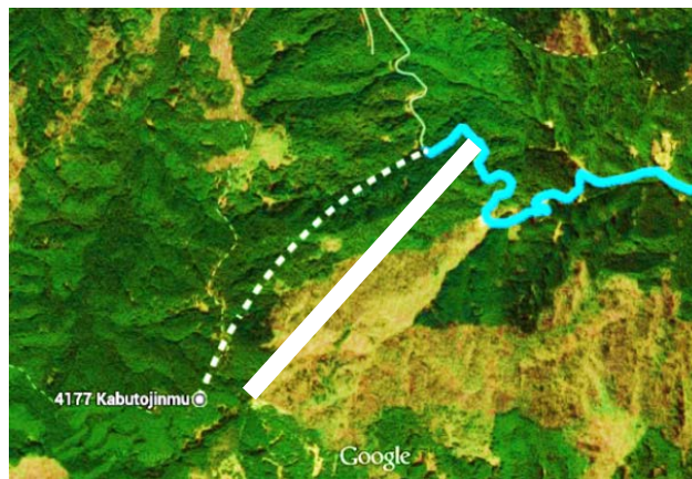
Figure 2 Accessibility measurement by Google Maps API. Blue line were measured based on the database of Google Maps. The part of white continuous line were measured as Euclid distance.
