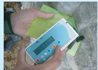
Measuring trend/plunge of a linear structure
