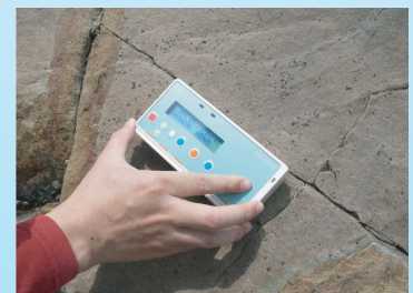
Measuring trend/plunge of a linear structure
